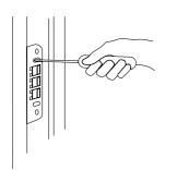
the door leaf align with the frame, the striking plate might need to be adjusted. The interior part of the striking plate is moveable and can be adjusted according to depth by loosening both
